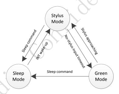
In stylus detection state, GT9110P will only detect stylus input. Finger touch is invalid.
