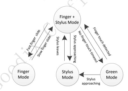
In auto-transition state, if GT9110P wants to switch to stylus mode after the host has issued the charge command, it is required that no finger touch should be present. The diagram below provides details:
