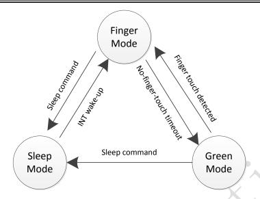
In Finger detection state, GT9110P will only detect finger touch. Stylus input is invalid.
