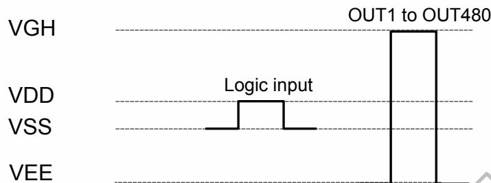
The logic levels of CPV, L/R, OE1, OE2, OE3, /XAO, MODE, STV1 and STV2 have to swing between VDD for "H" and VSS for "L".
