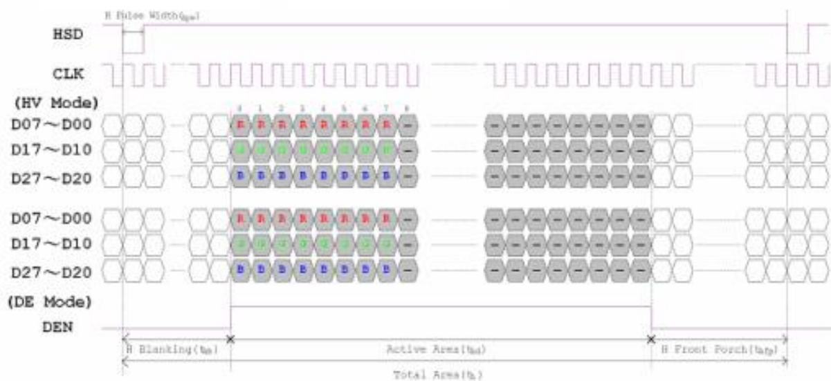
Figure 3.2 Horizontal input timing diagram.
