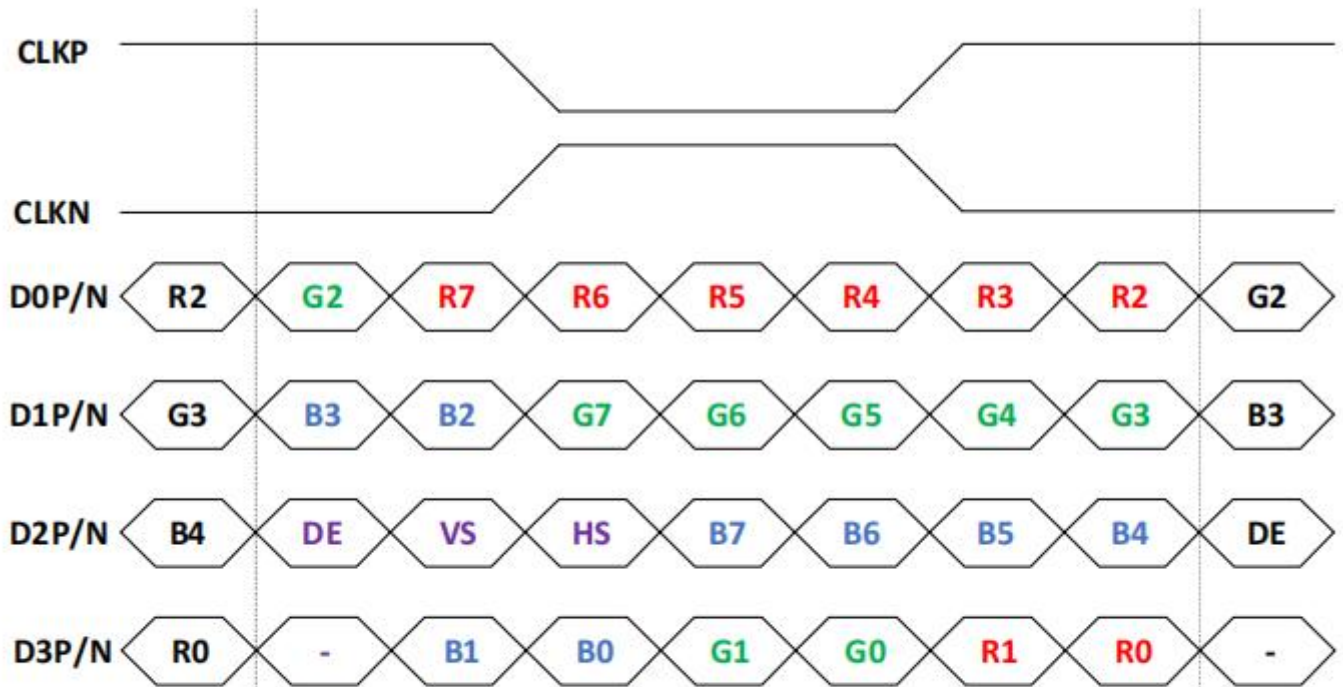
Figure 6.11: 8-bit LVDS input ( IM[1:0]=01, LANE[1:0]=11, LVFMT=1(JEIDA) )
